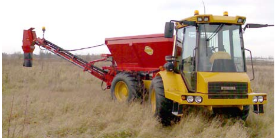
Here the previous model, 912C Series 2 with MultiChassis, mounted with a Bredal K65 sand distributor.
